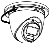
Figure 2-46 Snap the Camera into the Gang Box
