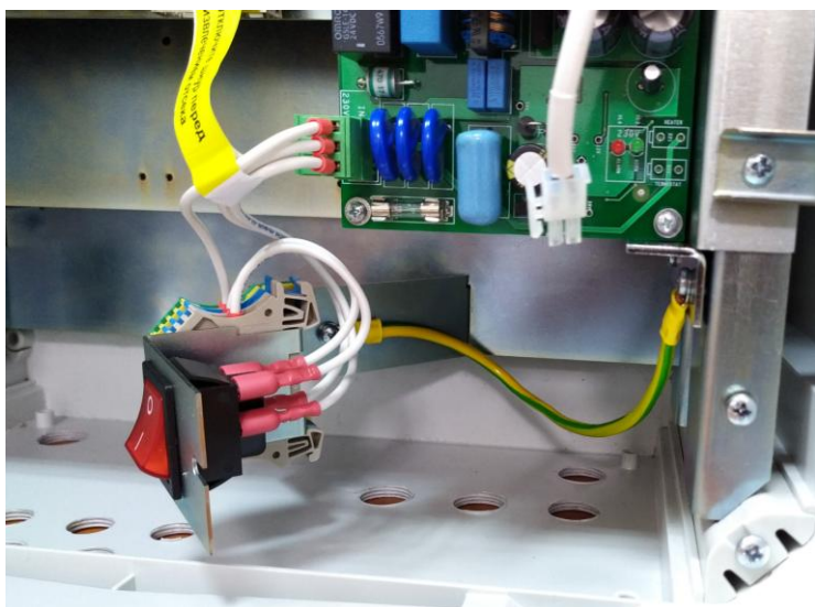
Figure 3.5.2 – Power supply unit with removed fastener.
